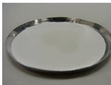
(Before measurement) 1 g of milk was dripped on to a fiberglass sheet for liquid measurements.
