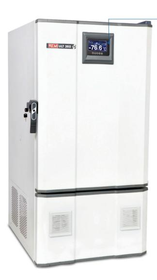
REMI's new range of Ultra-Low Temperature (ULT) freezers are specially designed for faster temperature pull down & optimized cryopreservation. Highly sensitive microprocessor control ensures precise temperature management at -86 °C. Recommended Ambient Temperature < 27°C.
